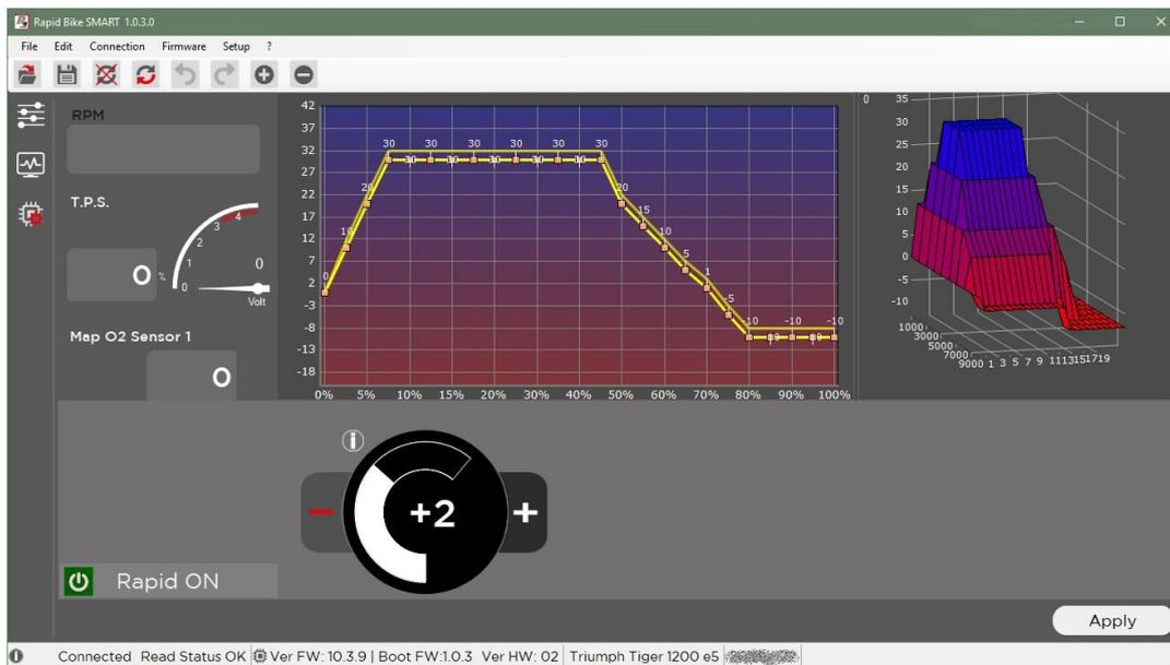
To connect with the SMART control unit, you only need an internal or external Bluetooth adapter for Windows PC/laptop at least release **4.0 BLE**. More information on the “Rapid Bike SMART” software manual, available in \Documents\SMART folder with its installation.
