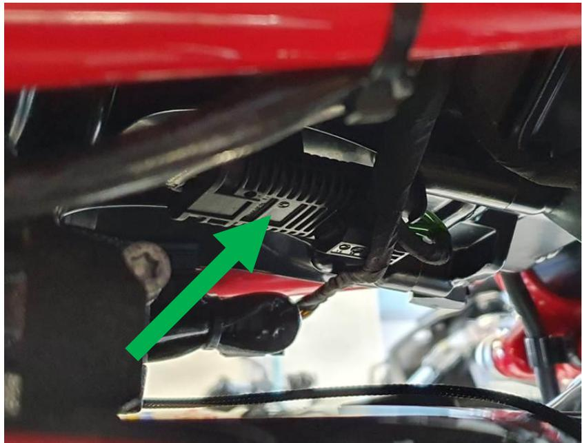
**Type:** 5 pins black plug, for cylinder/cylinders Lambda sensor (Wideband O2).
