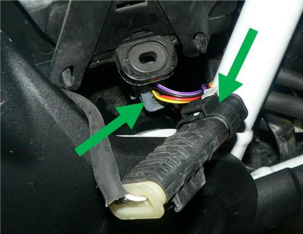
**6.4** Fasten all cables to the frame using zip ties.
