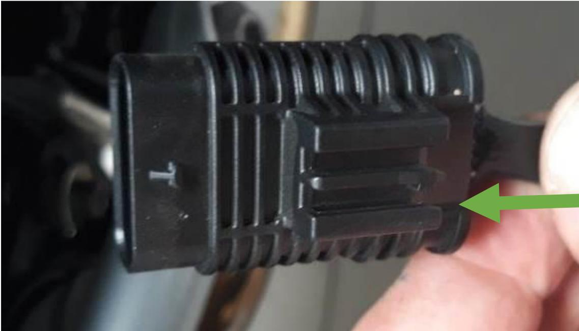
**6.2** Pull out and then push down the grey tab to disconnect the connectors.
