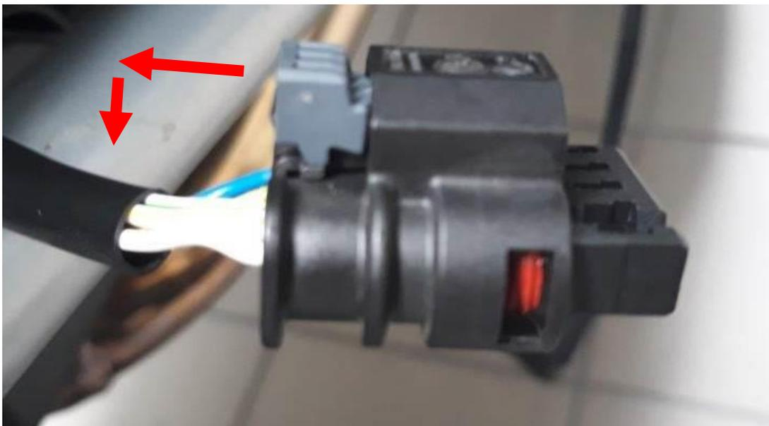
**6.3** Plug the connectors marked as **LW1** in-line with the stock wiring
