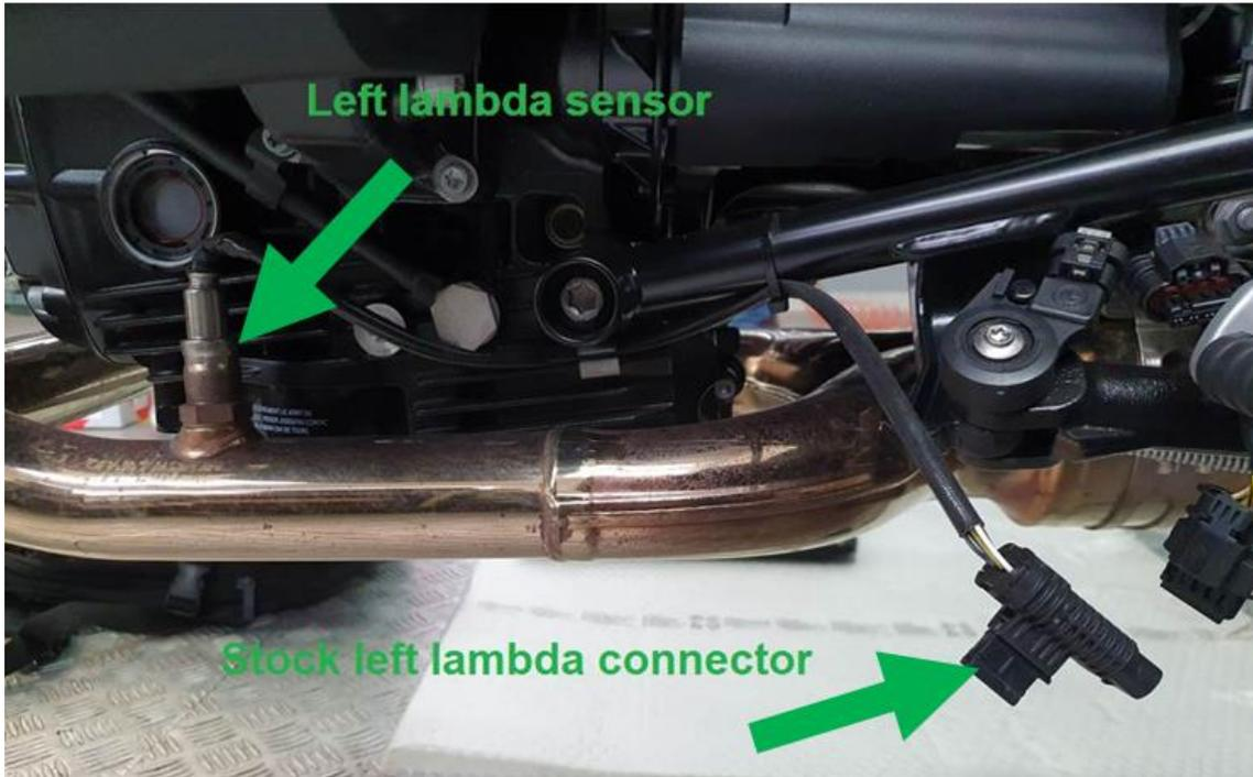
6.3 Plug the connectors marked as **LW1** in-line with the stock wiring
